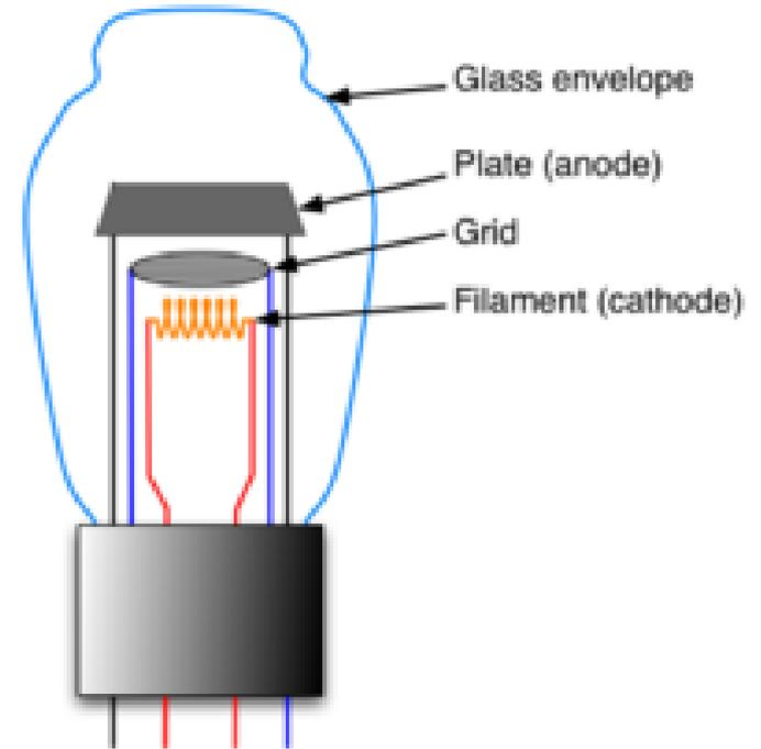
The resulting negatively-charged cloud of electrons is called a [space charge](#). These electrons will be drawn to a metal plate inside the envelope, if the plate (also called the [anode](#)) is positively charged relative to the filament (or [cathode](#)). The result is a flow of electrons from filament to plate.
